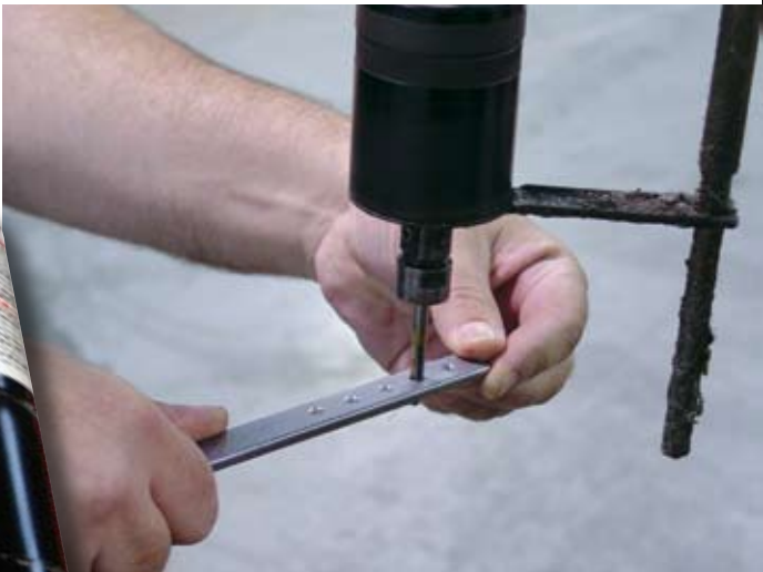
Automatic tapping machines extend tap life.
